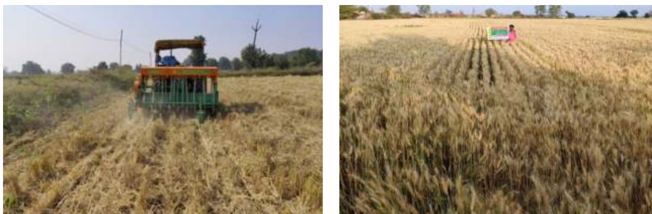
Fig. 1: Sowing of wheat with happy seeder and zero tilled wheat crop (WB 2)
