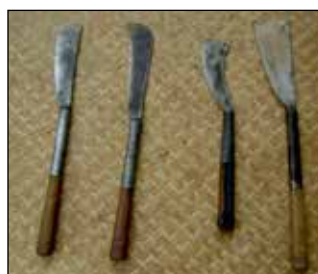
Figure 4a. Naga-Dao (Lepok) Field Capacity: 8 m 2 h -1 to 12 m 2 h -1
