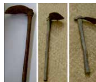
Figure 4b. Choktchü (Spade) Field Capacity: 10 m 2 h -1 to 15 m 2 h -1
