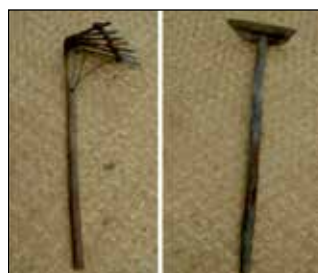
Figure 4c. Kheya (Bamboo and Wooden) Field Capacity: 15 m 2 h -1 to 20 m 2 h -1
