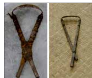
Figure 4d. Ehe (Hand Weeder) Field Capacity: 10 m 2 h -1 to 12 m 2 h -1
