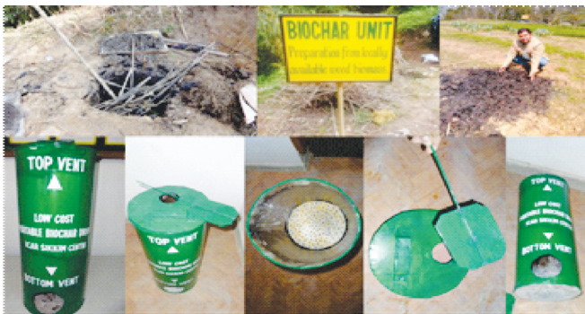
Figure 1. Biochar preparation technology by drum (kiln) and pit method
