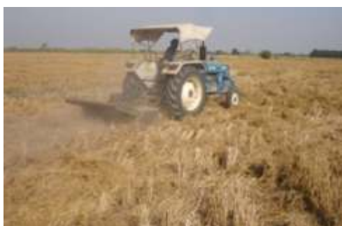
Fig. 1. A view of operation of tractor operated stubble shaver in combine harvested paddy fields
