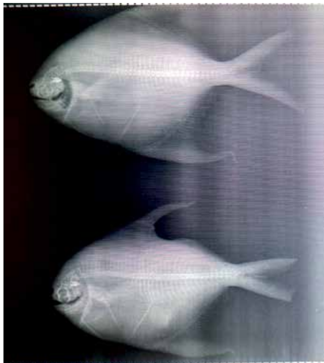
Fig 2. X-Ray radiograph of normal and abnormal specimen (showing SBS)
