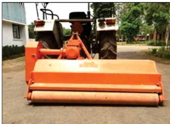
Fig. 1: Stationary view of tractor operated paddy straw mulcher
