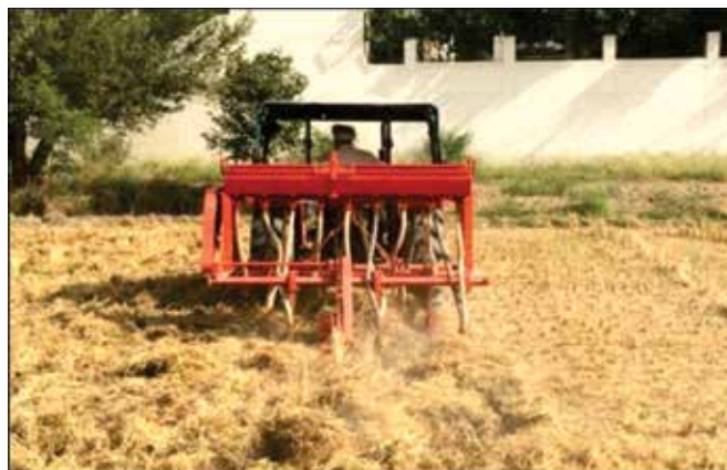
Fig. 5: View of wheat sowing being done in chopped straw field with spatial zero till drill.
