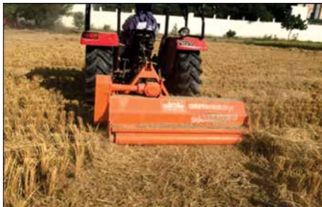
Fig. 4: View of tractor operated paddy straw mulcher in field.
