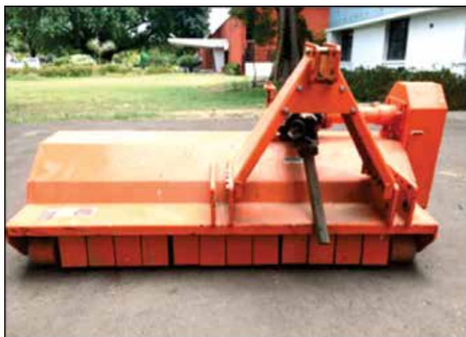
Fig. 1: Stationary view of tractor operated paddy straw mulcher
