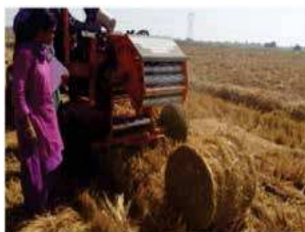
Demonstration of round type baler for densification of paddy straw
