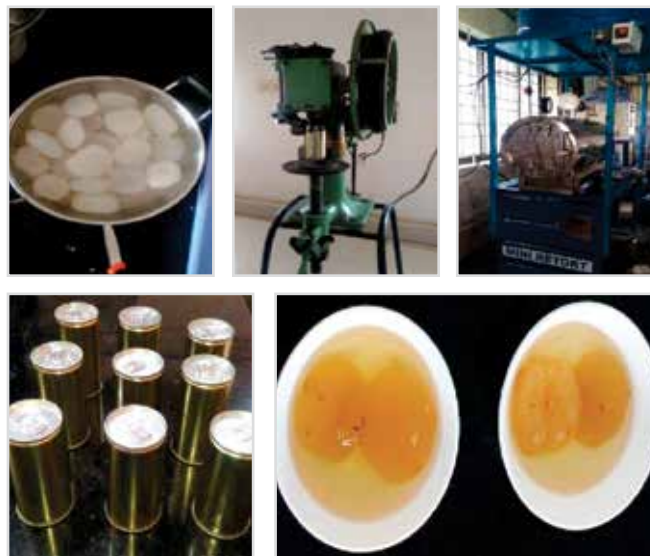
Fig.1 Process of canning: a) preparation of PTFE, b) filling and double seaming, c) heat processing of cans, d) after canning and e) finished product at 180th day
