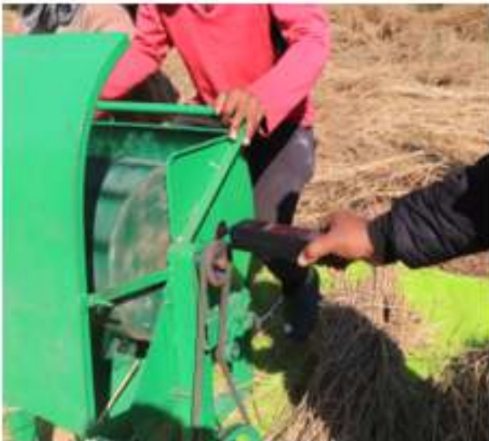
a. Measurement of cylinder speed by tachometer
